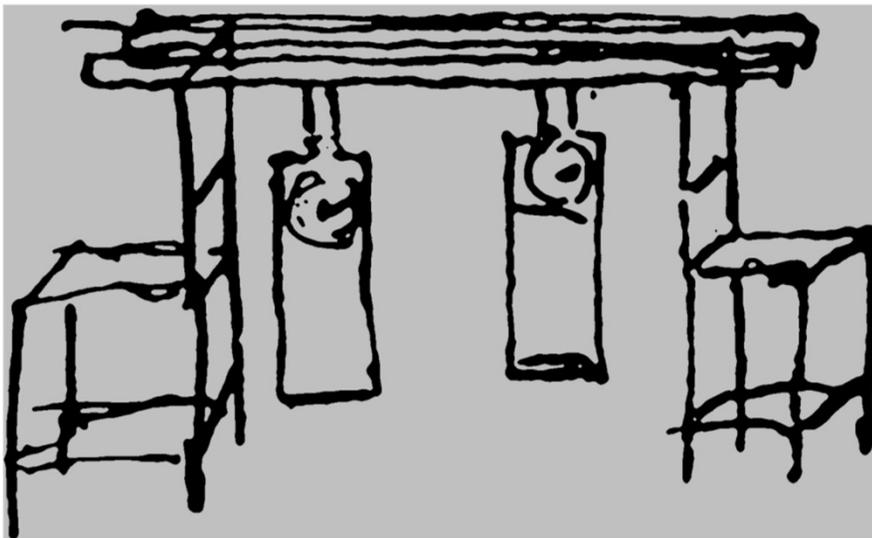
Two pendulum clocks hanging from a wooden support will transmit each other vibrations of very small intensity through the support. As a result, and this depending on other factors, the two clocks may start to oscillate at the same frequency, after some time
