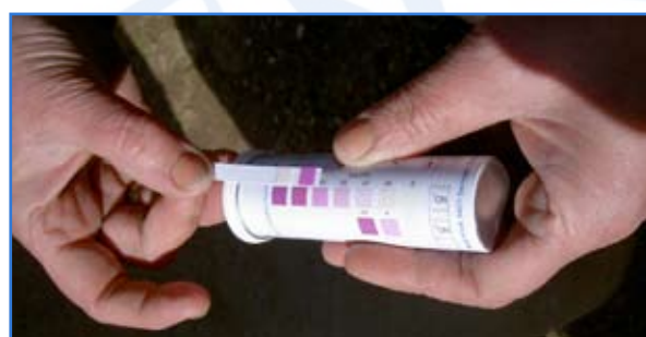
Fig. 4: Using nitrate quick tests ,and therefore nitrates can serve as an indicator for man-made (anthropogenic) water pollution Source: Margriet Samwel , WECF
