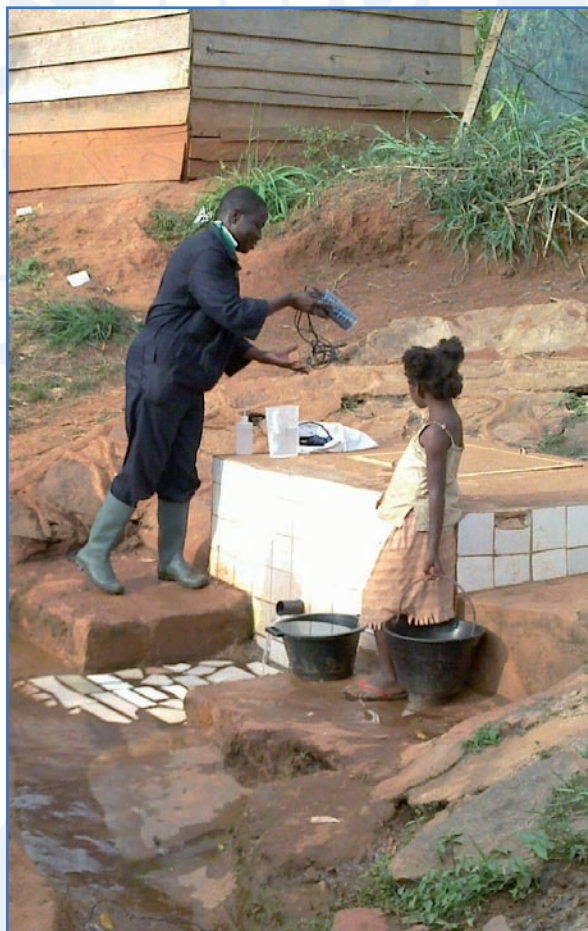
Figure 3: Sampling an amended and well maintained spring in Bastos, Yaoundé. Photo: Robert Kringel
