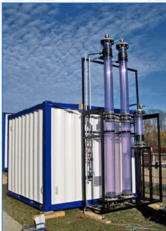
Figure 2: pilot Ozonation plant Source: S. Roder (RWTH Aachen University)
