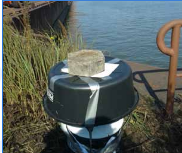
Figure 4: Mosquito trap with rain cover at the port of Hamburg Source: Kristina Militzer
