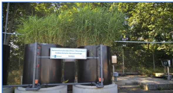
Figure 2: RSF test facility to investigate the effectiveness of RSF as an additional purification stage for WWTPs (Source: IHPH)
