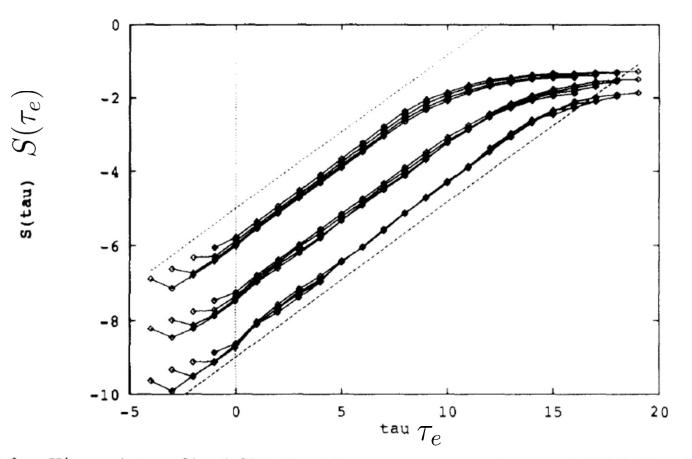
Fig. 2.  $S(\tau)$  for a Hénon trajectory of length 2000. The different curves correspond to  $\epsilon = 0.0005$ , 0.002 and 0.008 (the three bunches from bottom to top) and embedding dimension m = 2-5. The dashed lines have slopes  $\lambda_{\text{exact}} = 0.4169$ . Again  $\tau \leq 0$  corresponds to the components used to define the local neighbourhoods.
