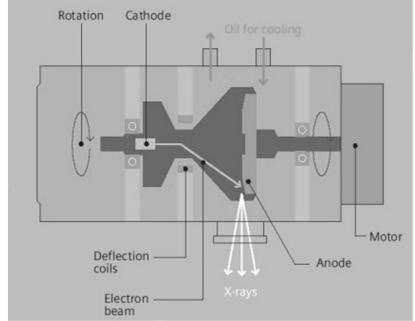
direct cooling of anode mechanics outside vacuum rotation time: 0.37 sec sub-mm volumen scans @ 500 mAs for 20 sec (64 mm/sec) dose reduction indep. of patient height and anatomy
