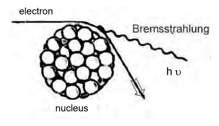
energy of Bremsstrahlung depends on trajectory of electrons
