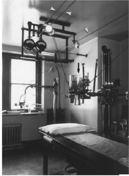
An x-ray examination room (Mayo Clinic, Rochester, Minnesota, circa 1925) with <u>bare high-voltage cables</u> (arrow-heads) and little shielding of the x-ray tube (arrow)
